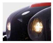
The **GEOTRAC 94** comes standard with powerful **bi-halogen headlights**. The 4 ellipsoid roof-mounted headlights provide reliable lighting when front equipment is attached.
