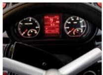
The central information board with I.B.C. display shows all vehicle information in one convenient place. In addition to RPM and speeds, various other functions can be called up. Pressing a button on the shuttle lever switches between daily operating hours, battery voltage or fuel consumption display.
