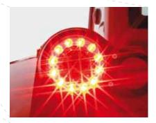
**LED reverse lights** - Because light-emitting diodes have an extremely long life up to 20,000 operating hours, reverse and brake lights last virtually the entire life of the tractor itself and are nearly maintenance-free.
